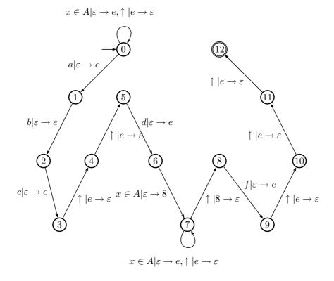
Figure 3. Pattern matching PDA for tree pattern shown in Figure 2
